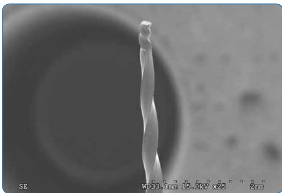
Figure 4 - SEM image of the separated file tip. An 180° unwinding can be seen near to the point of fracture.
