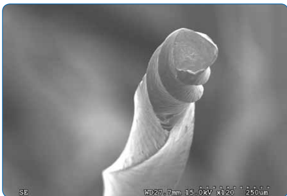
Figure 5 - SEM image of the separated file tip. Another vision of the unwinding area near to the point of fracture.
