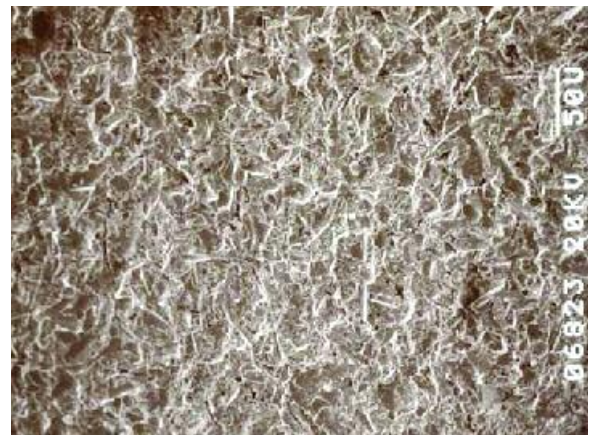
Figure 4 - SEM micrograph of the amalgam surface after aluminum oxide airborne
