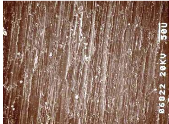
Figure 3 - SEM micrograph of the amalgam surface roughened with a greenstone
