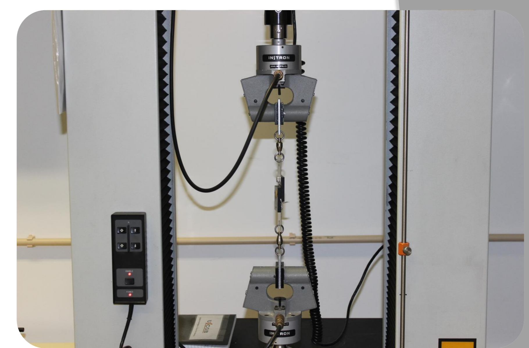
Figura 3 - Máquina de testes Universal Instron (Instron Ltd, Bucks, HP123SY, England)
